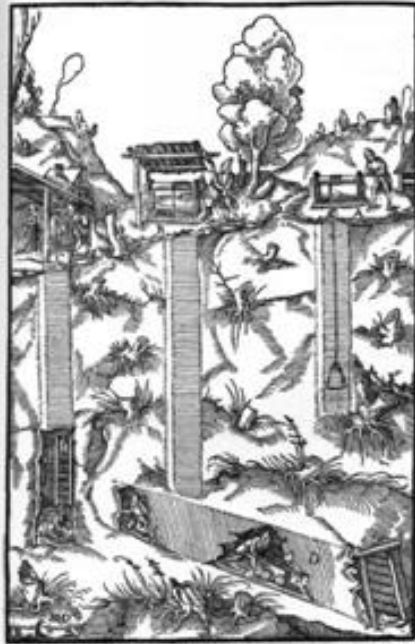
THREE SEVERAL DEPTHS, OF WHICH THE FIRST, A, DOES NOT REACH THE TUNNEL, THE SECOND, B, REACHES THE TUNNEL, IN THE THIRD, C, THE TUNNEL WAS NOT THE DEEPER. (B-TUNNEL)
