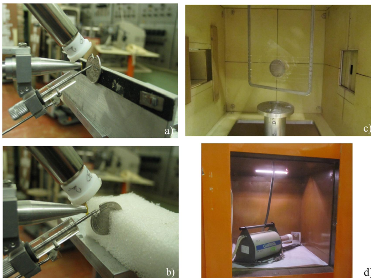
Fig. 1: Experiment photos. a-b Using PIXE the middle part of both platinum coins and the cut inner surface was analysed with a 1.5 mm diameter beam. c During the PGAA measurements, nearly the entire volume was irradiated in the NIPS-NORMA sample chamber. d The off-line counting measurements after the neutron irradiation took place at the low-background chamber.
