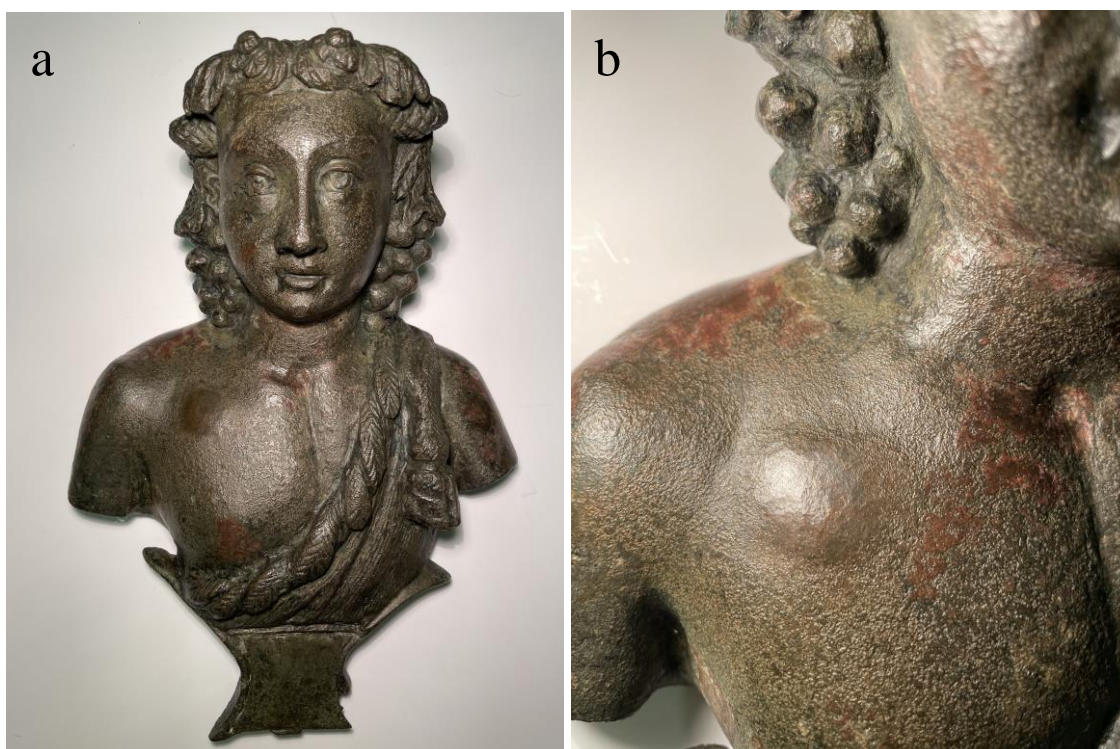
Fig. 7.: Bacchus bust (HNM n. 3.1944.) a – The alloy is Cu with 6,7 weight% Sn and 18 weight% Pb. The bust still retains most of the natural patina, covered by conservation resin. b – The ancient repair (Cu with 6.2 weight% Sn and 7.6 weight% Pb) on the right side of the bust, under the natural patina, was evidenced with raking light for the photo. (Photo A. Giunlia-Mair)
