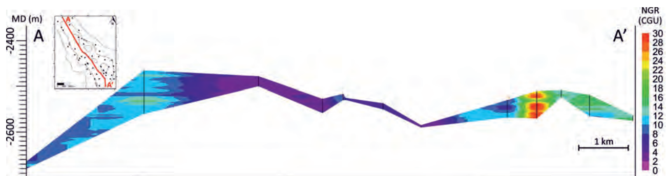
Figure 4. NW–SE cross-section across the Algyő High displaying the distribution of natural gamma-ray intensity (NGR) [Conditional Gamma Units (CGU)] values. Black lines indicate the locations of boreholes. The point map of the area illustrates the A–A' cross-section line and the wells with NGR [CGU] data. The vertical scale of the cross-section is exaggerated 2×. MD: measured depth
