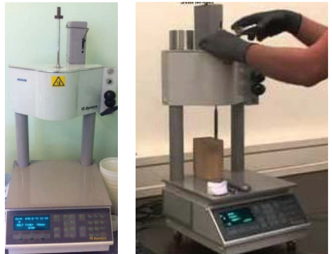
Fig. 5. Dynisco capillary rheometer (left) and the viscosity measurement of feedstock (right)
