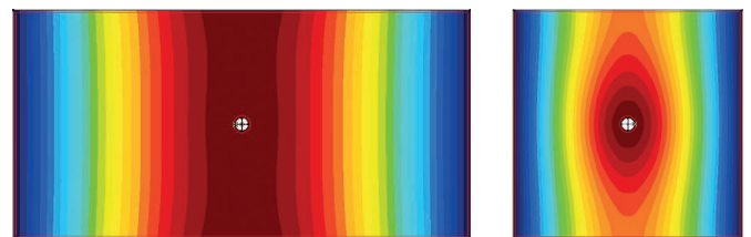
Fig. 7 Left: 6 mm, 360×860 mm glass table deformation. Right: 6 mm, 360×460 mm glass table deformation
