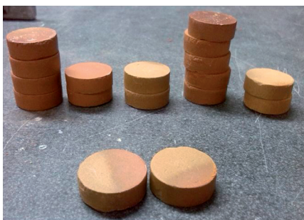
Fig. 4. The sintered at 1250°C ceramic disc specimens with different volumes of Al 2 O 3 and ZrO 2 powders in the raw material mixtures
