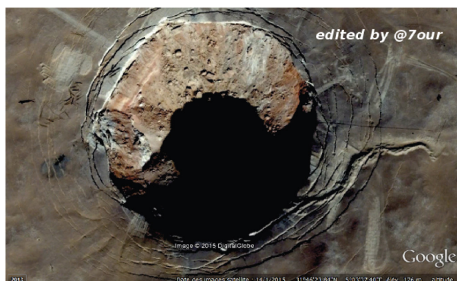
Fig. 1. Satellite photo of 14 January 2015 showing Haoud Berkaoui crater with a diameter of approximately 350 m (Credits: Google Earth)
