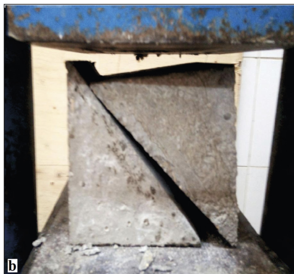
Fig. 9. a) 5% EPP mortar sample shows interface failure with partial damage and attached traces of substrate (right), b) interface failure with complete separation
