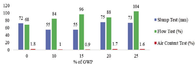
Fig. 3 Results of slump, flow table and air content tests (25MPa Concrete Mix)
