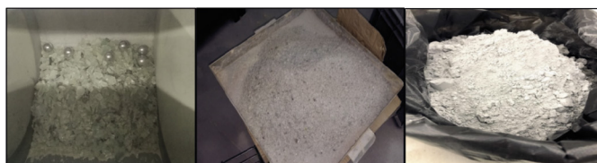
Fig. 2 Glass particles reduced from 30 mm to less than 75 µm
