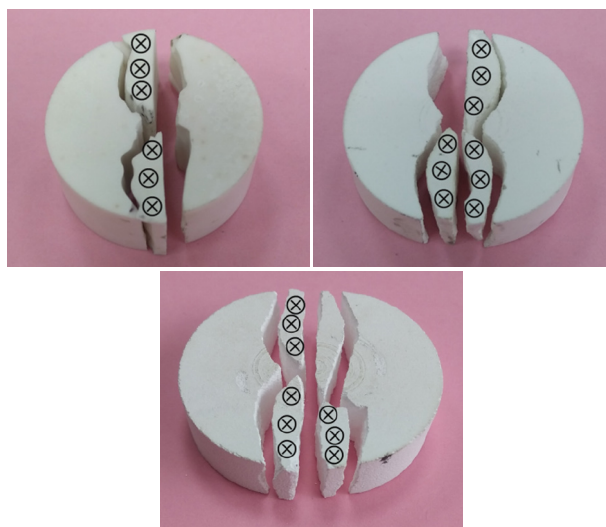
Fig. 5 Macro photographs of samples with different porosity (a - 4% ; b - 17% ; c - 42%) after diametral compression tests with XRD schemes
