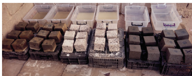
After immersion in a solution of 5%Na 2 SO 4 After immersion in a solution of 5%H 2 SO 4 After immersion in fresh water
