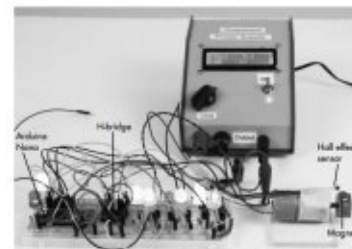
Figure 4-4: The Watch Winder breadboard was used as a proof-of-concept for the project. Here, I powered it with the Regulated Power Supply from Chapter 3.
