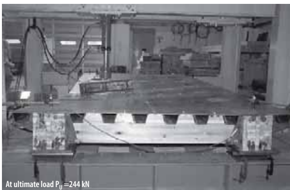
Fig. 9 Bridge model shown during loading
