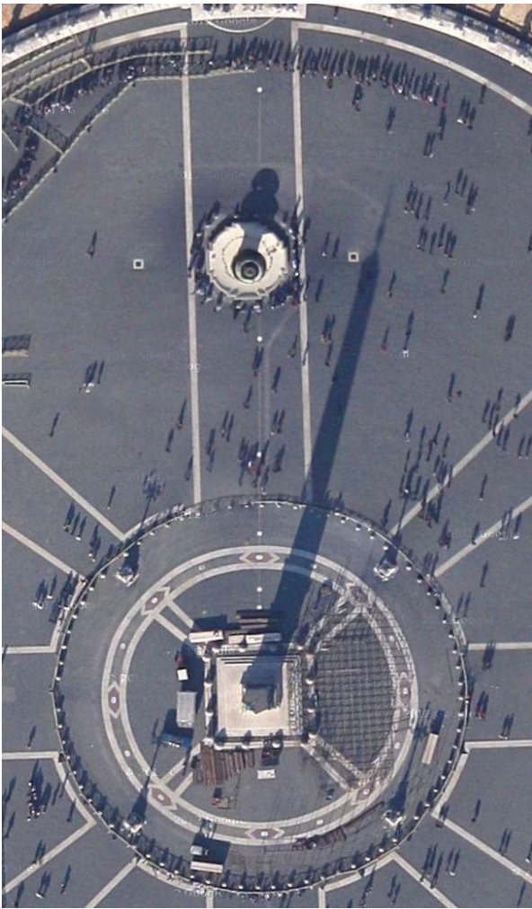
The obelisk of St. Peter's Square in Google Earth. The meridian line and markers are well visible, (and the slight inclination of the axis of the square to the East-West direction), also the 16 markers of the compass rose, with the wind directions
