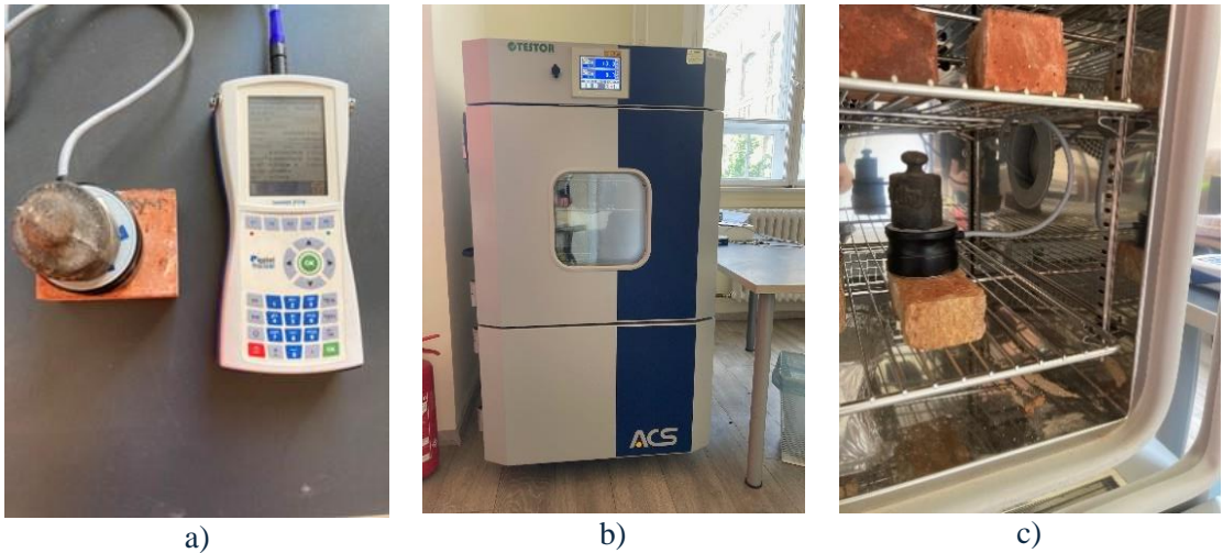
Figure 3 Tools of thermal characterization: a) MTPS probe, b) climatic chamber and c) sensor installation
