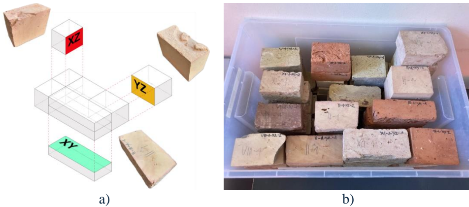
Figure 1 a) Creating of different planes of samples and b) all samples of different masonry bricks
