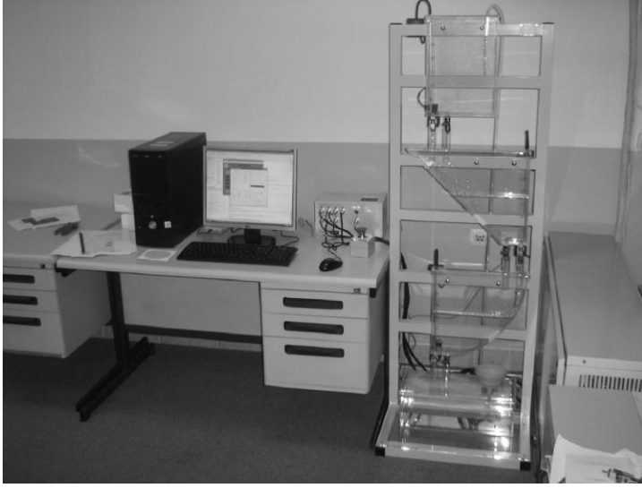
Figure 2 The multitank system by Inteco
