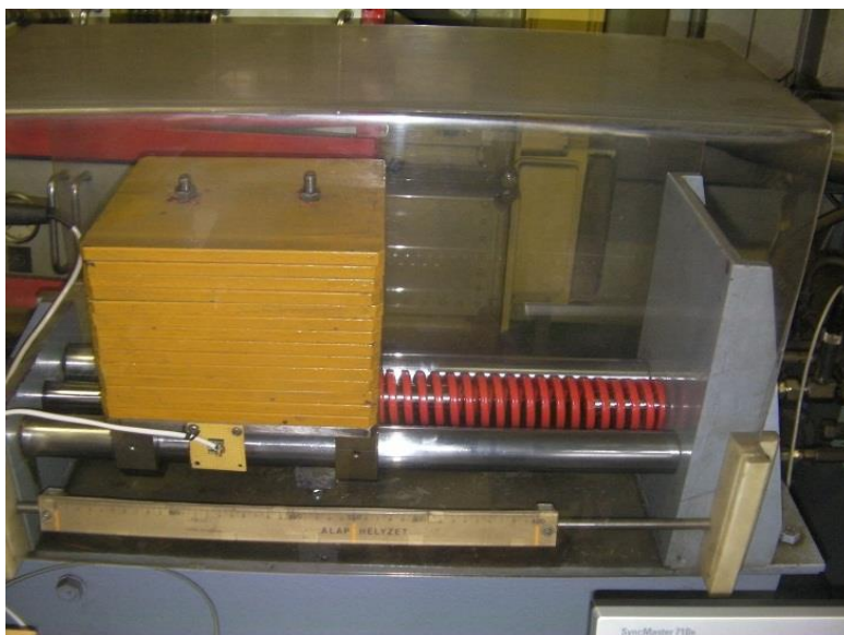
Figure 10 Mass-spring mechanical load of the positioning system
