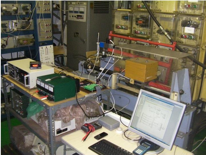
Figure 8 Electrohydraulic positioning system and computer control
