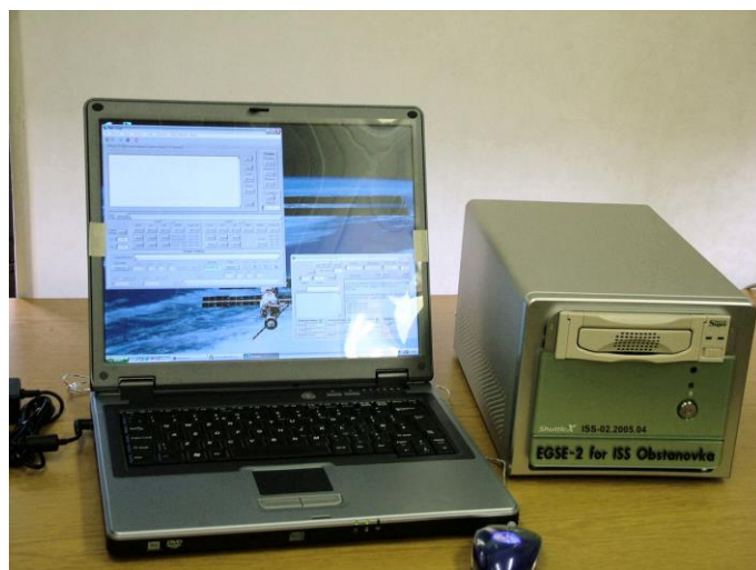
Figure 12 Photo of realized EGSE of Obstanovka
