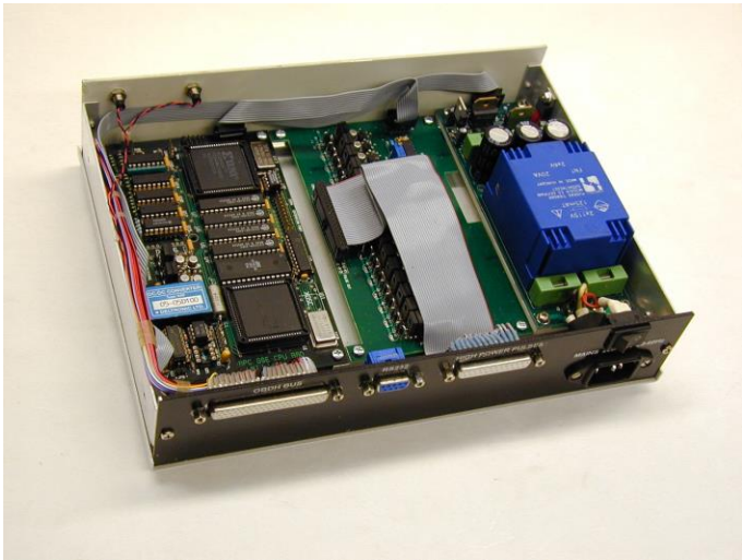
Figure 6 Photo of the realized EGSE
