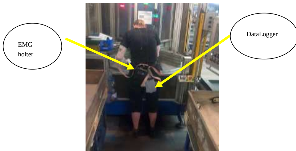
Figure 6 Measuring in factory: dependency between the EMG measurements and the muscle force recorded by datalogger: Operator in ITT holding Ostrava (own processing)
