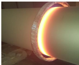
Figure 2 Inductive remelting process of the NiCrBSi coating
