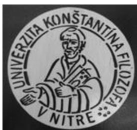
Figure 4 Example of engraving image on stainless steel plate
