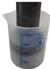
Figure 6 Shredded PET volume reduction test
