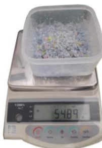
Figure 5 Consistency of the shredded PET bottles
