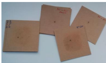
Figure 6 Samples of the transformerboard used for model evaluation
