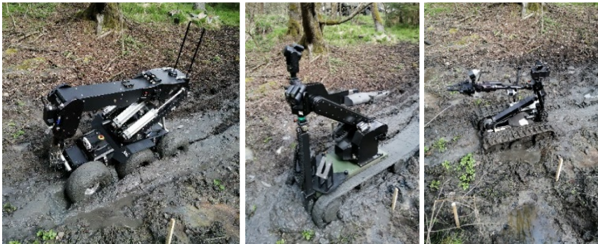
Figure 9 Robotic devices Tallon, Defender and tEODor mired in the terrain
