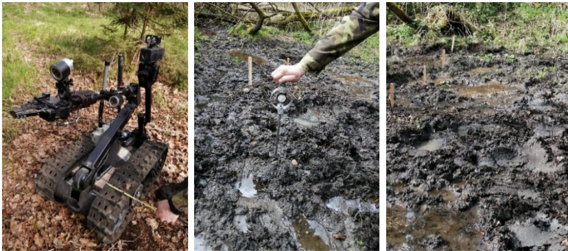
The marked low endurable terrain, measurement with cone penetrometer and measuring of the features of robotic device
