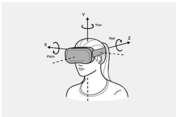
Figure 8 Oculus Quest 2 coordinate system [11]
