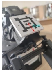
Figure 8 AprilTag's position on the robot
