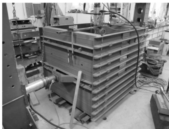
Figure 8. For the tests prepared multi-level shear box [17]
