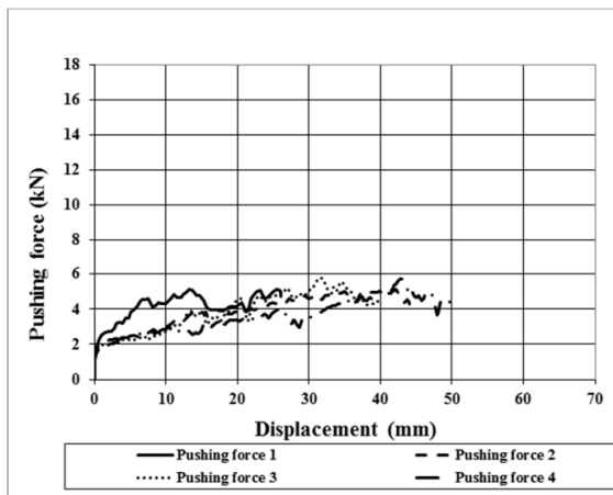
Figure 14. Pushing force-displacement diagram, compacted layer structure with geocomposite type 1, shearing plane Nr. 4. [17]
