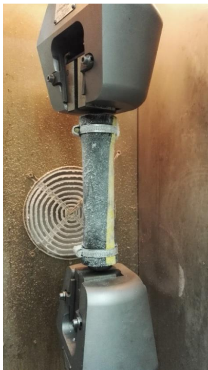
Figure 12. Hose piece specimen at -40 °C, placed in climate chamber
