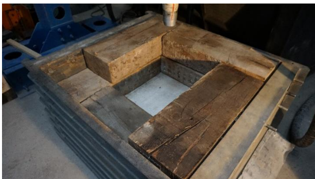
Figure 3. The wooden sleepers in the shear box
