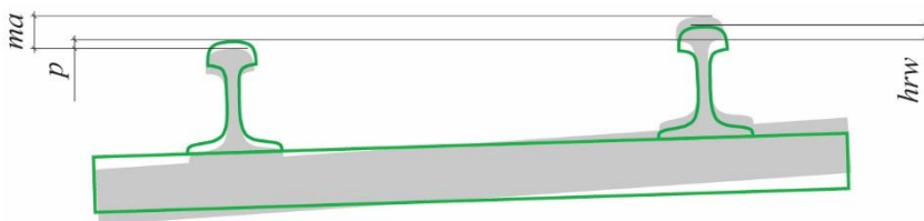
Figure 7. The first boundary condition (in this and subsequent Figures, the existing position for assembled rails and sleepers are shown in gray solid color, the calculated position is in green)
