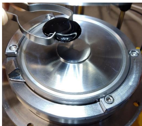
Figure 3. Putting a 25 mm diameter specimen onto the DSR plate
