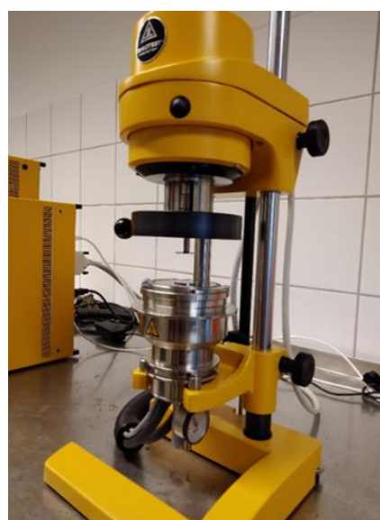
Figure 1. Dynamic shear rheometer (DSR), Rheotest 4.3
