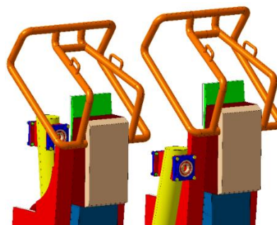
Figure 7. Restraint system of the gondola
