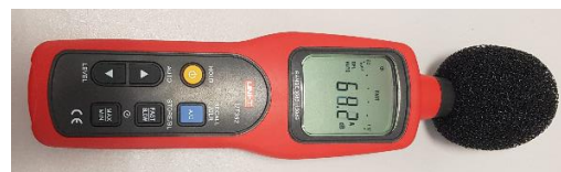
Figure 6. Used UT352 digital noise level measuring instrument, source: own photo
