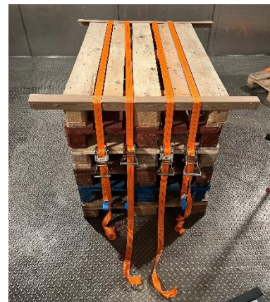
Figure 8. Lashed dummy load
