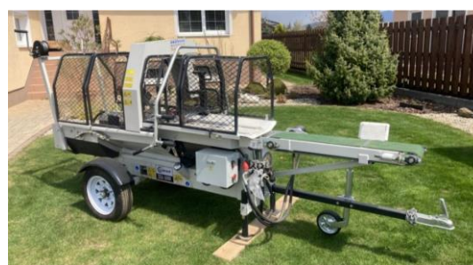
Figure 1. A solved mobile working machine with additional input belt conveyor
