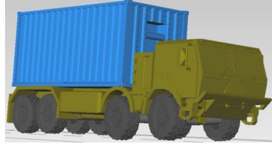
Figure 6. The created multibody model of the solved off-road lorry
