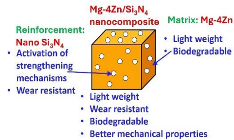
Figure 2. Using \text{Si}_3\text{N}_4 nanoparticles to improve wear properties of Mg-4Zn alloy
