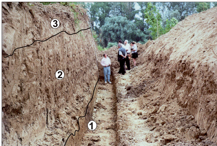
Photo 1. Section South from Szolnok with intense floodplain sedimentation. – 1 = alluvial meadow soil formed prior to flood control; 2 = 200–230 cm thick siltation; 3 = 30–40 cm thick sediments deposited between 1986 and 2000. (Photo by SCHWEITZER, F. 2001)
