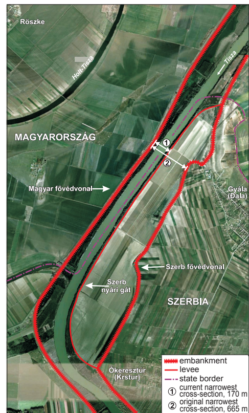
Fig 5. Shrinkage of active floodplain of Tisza in Serbia due to the construction of levees (eds: NAGY, I. and SCHWEITZER, F. 2011 by using Google Earth images)
