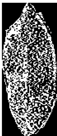
Figure 12. Image of an overexposed leaf object. White and gray areas indicate pixel intensity between 230 and 254, black areas indicate pixel intensity 255 or over.
