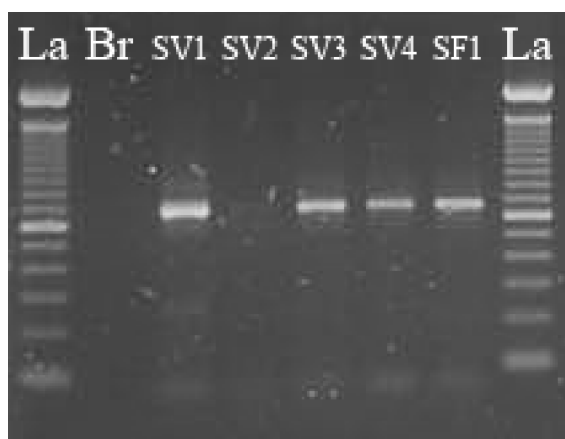
Figure 2. A 1,5 % agarose gel including a 100 bp ladder (La) and the negative control (Br). Fragments of 650 bp correspond to the amplification product of the PC-IGS from samples of cyanobacteria blooms from São Francisco Verdadeiro (SV1, SV2, SV3 and SV4) and São Francisco Falso (SF1) tributaries, using the PC \beta F and PC \alpha R primers
