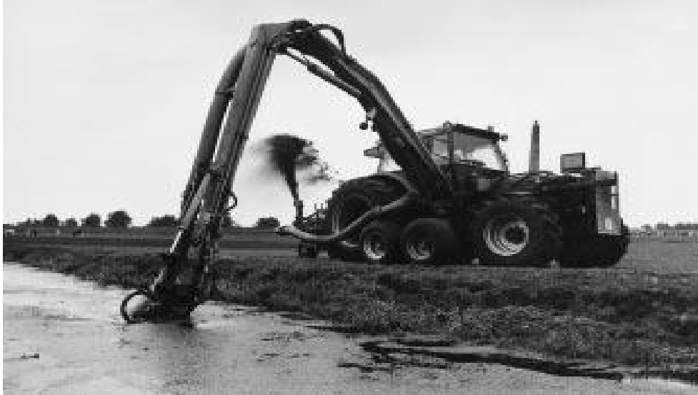
Figure 6. An example of a dredging machine, the suction-pipe. This removes mud from the ditch by hanging a hose in the mud through which the mud is sucked up and sprayed in a wide range over the adjacent field (From Twisk et al., 2000)
