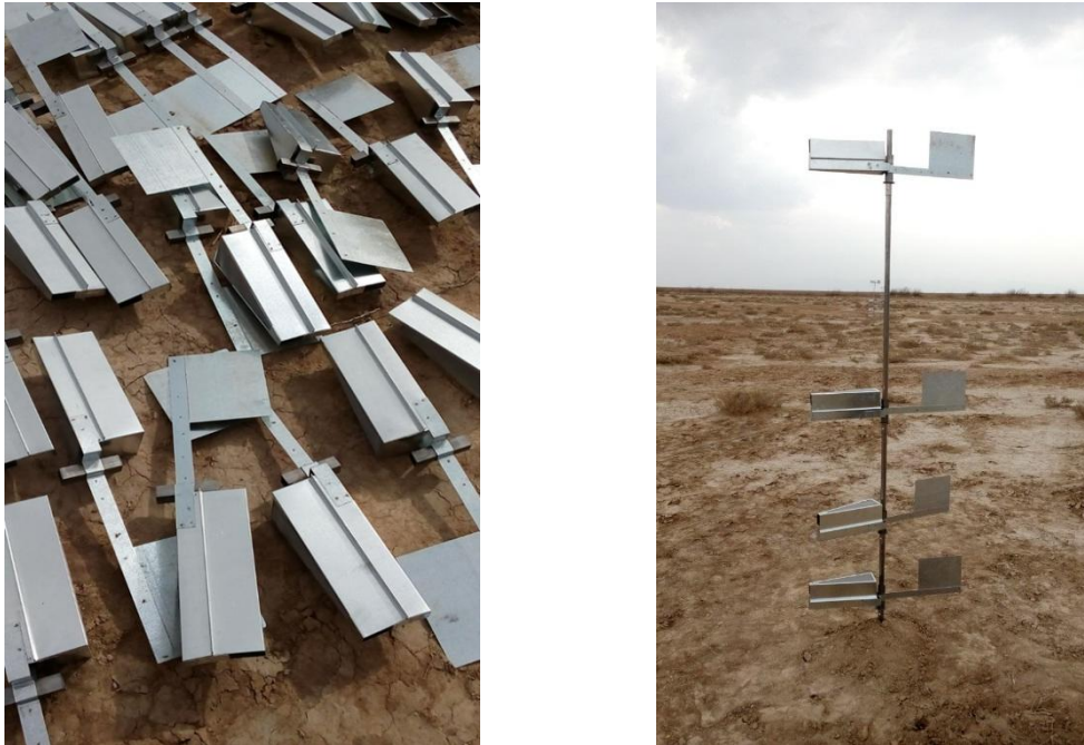
Figure 3. Samplers that were made and installed
