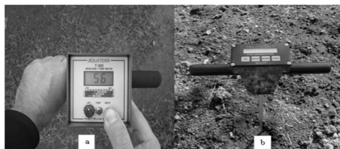
Figure 3. Soil moisture and temperature measurement instrument (a) and soil penetrometer (b)
