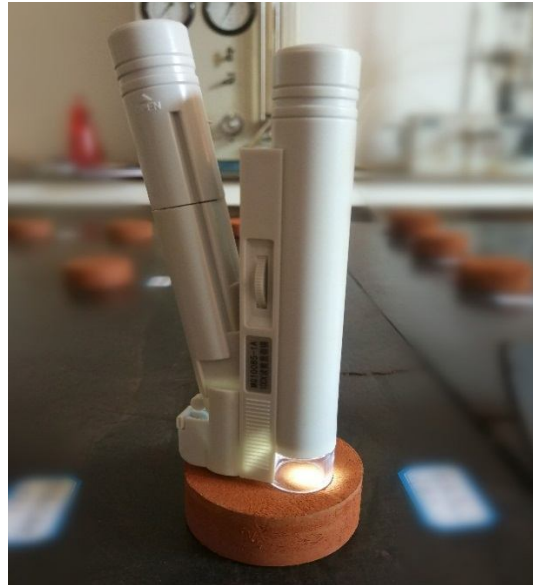
Figure 2. The visualizer of crack width (100x)
