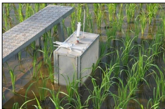
Figure 2. The closed chamber method was used to collect gas samples for determining nitrous oxide flux
