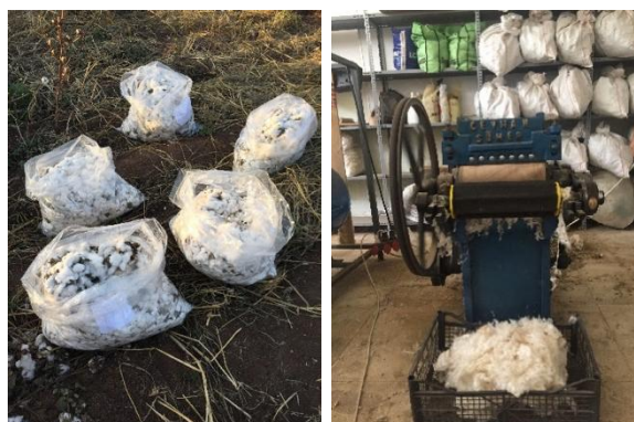
Figure 3. Samples of cotton and the ginning process of the seed cotton
