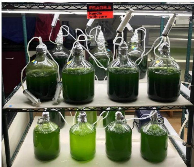
Figure 2. Experimental set-up used for cultivating microalgae
