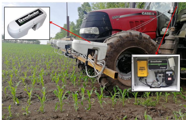
Figure 3. Ground-based remote sensing detection system for the acquisition of maize canopy NDVI data
