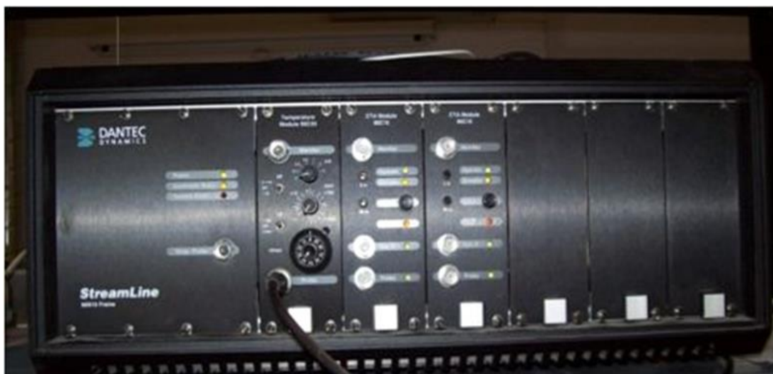
Figure 3. DANTEC CTA (Constant Temperature Anemometer)
